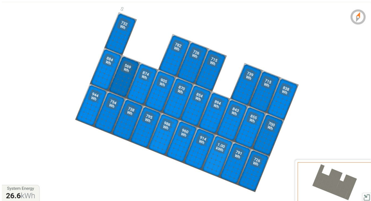
Rooftop solar array w/ microinverters (battery in garage), Enphase system
